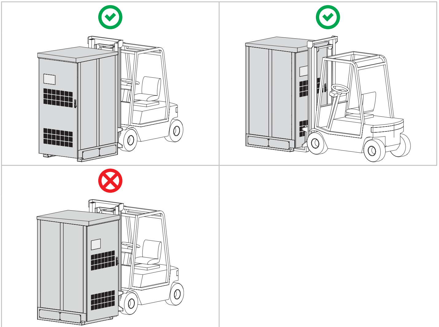
Figure 1 - Handling of the unit using pallet truck with 1.30m long forks (screen shall be at the back, if not possible it can be at the front, but then take care of the screen)
