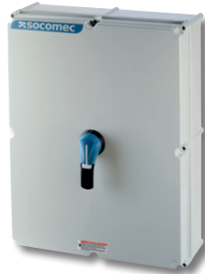
SIRCOVER enclosure 160 to 630 A Polyester - IP65
